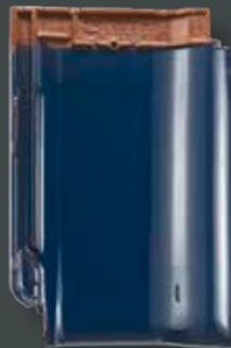
Our innovative production method, which fires the tiles upside down to save space, increases energy efficiency and ensures that colour only reaches where it is needed. Uncoloured fold areas disappear after covering by overlapping of the surrounding tiles. This way you can save resources and make roofs sustainable.
